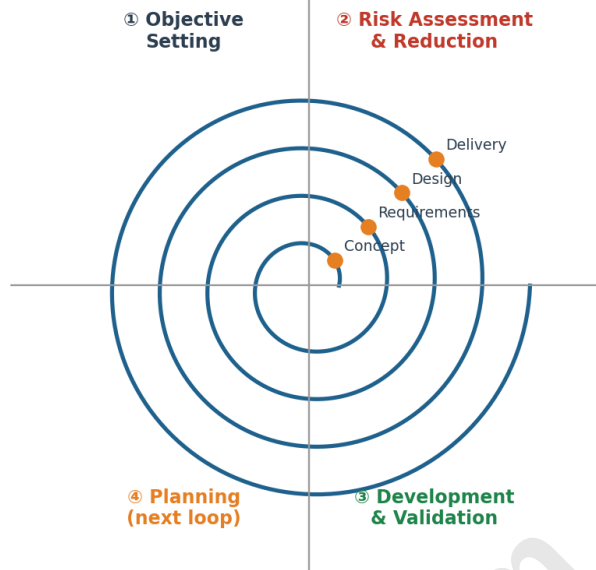
Figure 2.2: The spiral model – four sectors per loop
